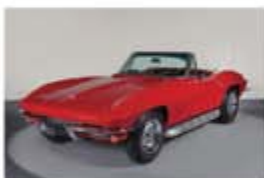
1967 CHEVROLET CORVETTE Numbers matching, 4-speed, highly desirable L79 option 327/350 engine
